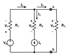
2. Connect the circuit in Figure 1. Record the exact values of V<sub>S</sub> and I<sub>S</sub>.
